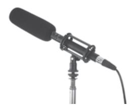
Shotgun microphones use a standard directional capsule, usually a super-cardioid, with a long, hollow, slotted interference tube attached to its front surface.
