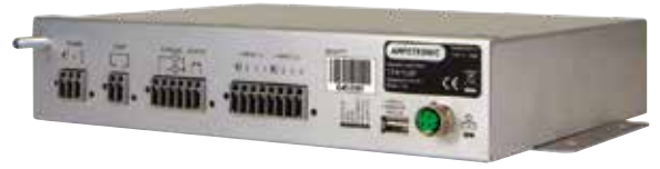
T14-1LB: 24V DC power, Wago connectors
